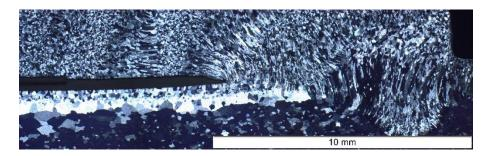
Macro grinding in cross-section through a layer structure with embedded layered stacks of Copper and Aluminium oxide structure (appearing as a black zone in the middle of the left half of the image)
